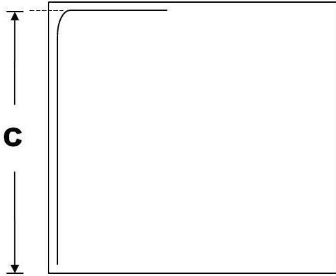
C = measurement from the floor to the roll up door track at the rear before the curve to the vertical door track
